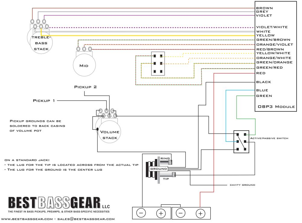
9 OR 18 VOLTS CAN BE USED WITH THE OBP2/OBP3 PREAMPS. FOR 9 VOLT USE, CONNECT THE NEGATIVE FROM THE BATTERY TERMINAL TO THE RING ON THE JACK.
