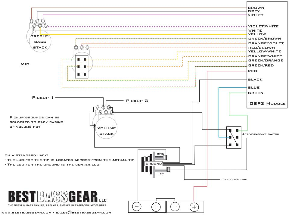
9 OR 18 VOLTS CAN BE USED WITH THE OBPZ/OBP3 PREAMPS. FOR 9 VOLT USE,
