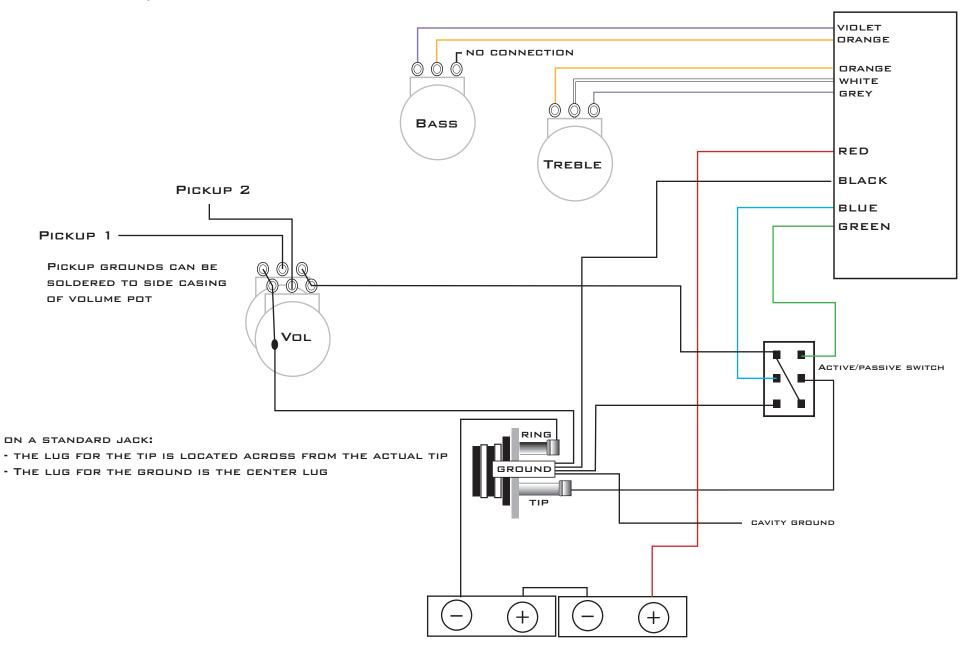
18 VOLTS IS TO BE USED WITH THE OBP1 PREAMPS.
