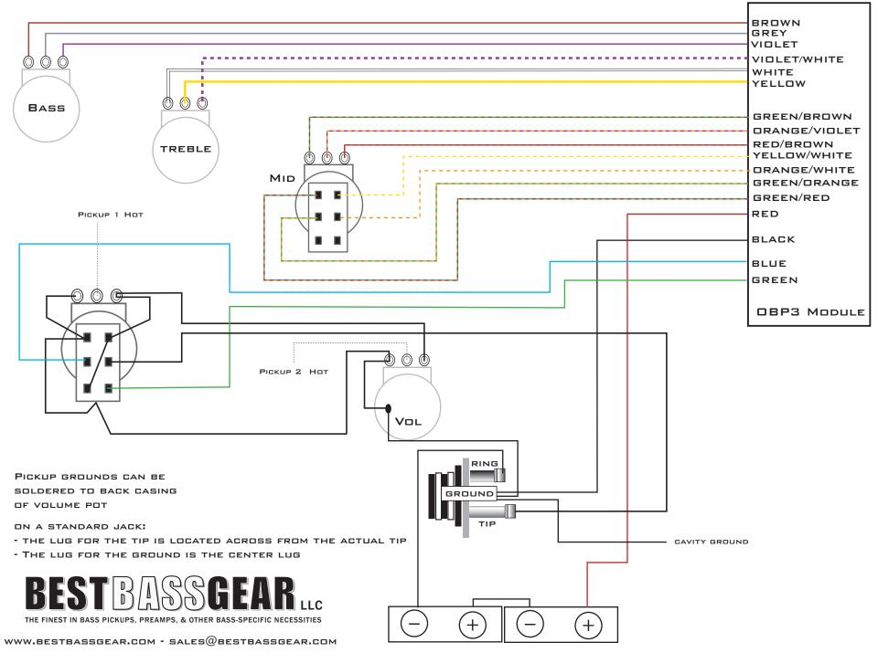
9 OR 18 VOLTS CAN BE USED WITH THE OBPZ/OBP3 PREAMPS. FOR 9 VOLT USE, CONNECT THE NEGATIVE FROM THE BATTERY TERMINAL TO THE RING ON THE JACK.
