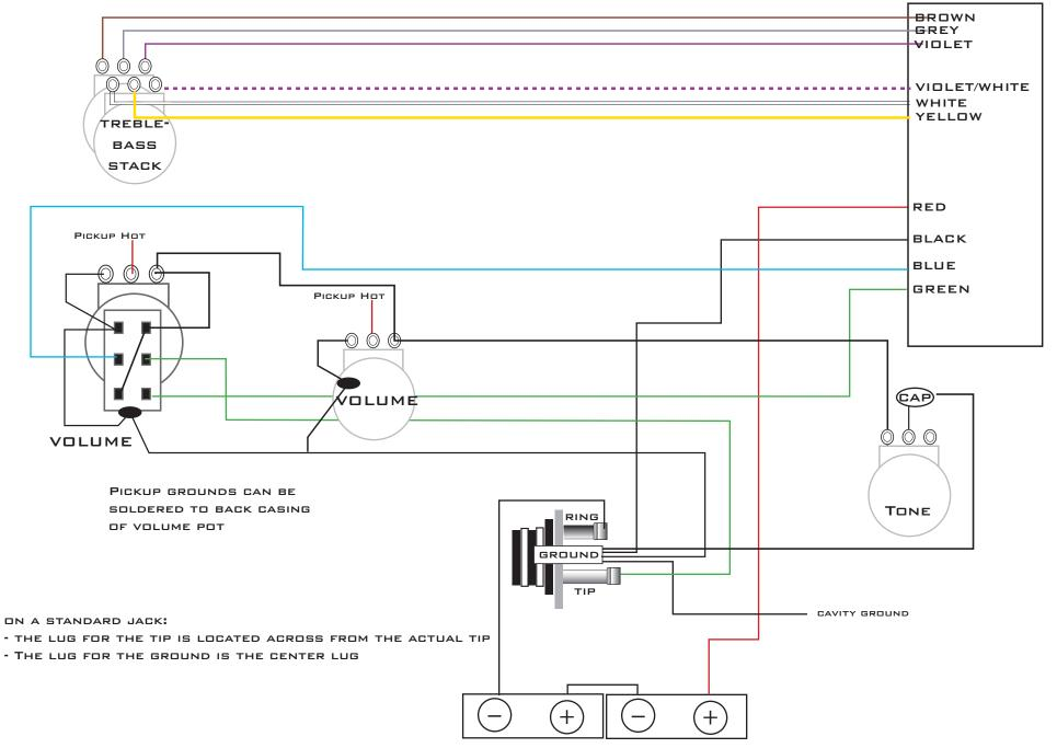
9 OR 18 VOLTS CAN BE USED WITH THE OBPZ/OBP3 PREAMPS. FOR 9 VOLT USE, CONNECT THE NEGATIVE FROM THE BATTERY TERMINAL TO THE RING ON THE JACK.
