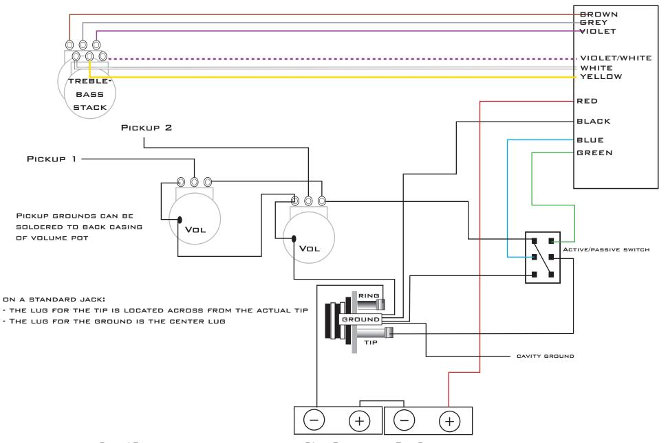
9 OR 18 VOLTS CAN BE USED WITH THE OBPZ/OBP3 PREAMPS. FOR 9 VOLT USE, CONNECT THE NEGATIVE FROM THE BATTERY TERMINAL TO THE RING ON THE JACK.
