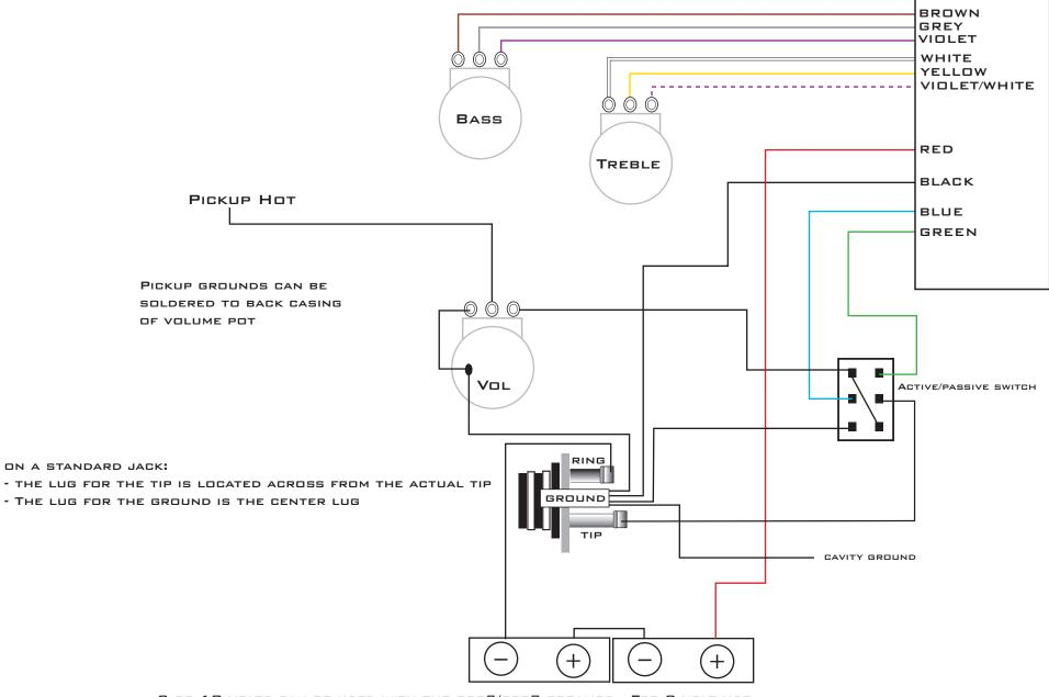
9 OR 18 VOLTS CAN BE USED WITH THE OBP2/OBP3 PREAMPS. FOR 9 VOLT USE, CONNECT THE NEGATIVE FROM THE BATTERY TERMINAL TO THE RING ON THE JACK.
