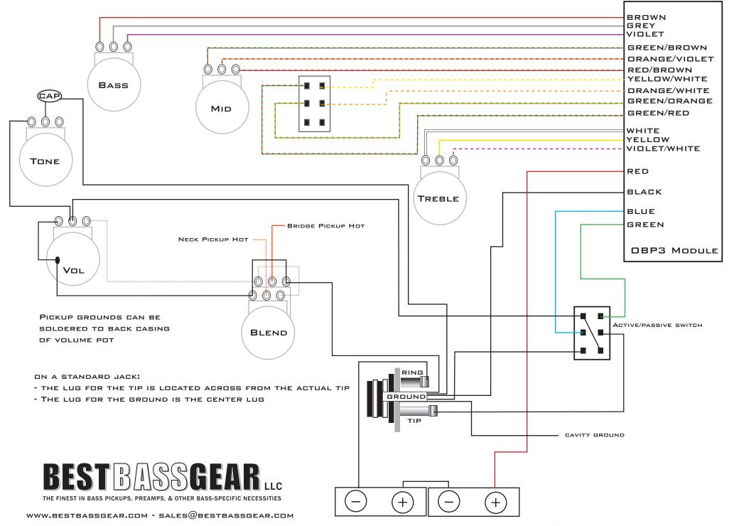
9 OR 18 VOLTS CAN BE USED WITH THE OBP2/OBP3 PREAMPS. FOR 9 VOLT USE, CONNECT THE NEGATIVE FROM THE BATTERY TERMINAL TO THE RING ON THE JACK.
