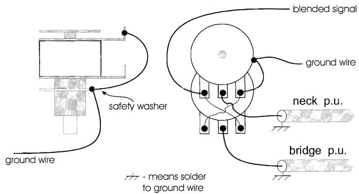
DO NOT OVERHEAT WHEN SOLDERING GROUND WIRES OR ANYTHING ELSE TO THE SIDE OF THESE BLEND POTS
