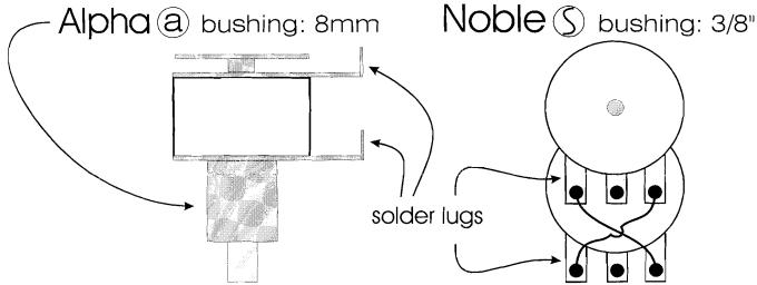
Blend pot wiring viewed from the inside of the control cavity (pot. shaft down)
