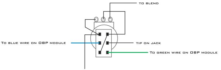
GROUND TO CASING ON VOLUME POT AND THEN ONTO JACK GROUND.
